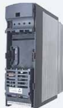
Location of EM-IO-03 module on the frequency inverter
